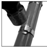
8. Hammer down buckle ears to hold band stub in place to complete BAND-IT clamp.
